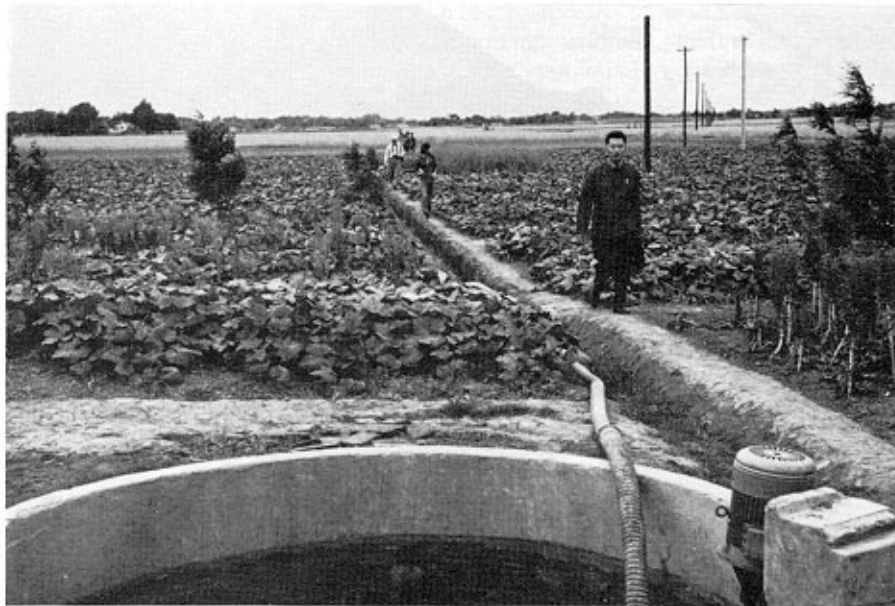
Plate 27. A biogas-driven pump removing effluent from a large biogas unit for direct field spraying. (Pin Niu People's Commune, Jiangsu Province).
