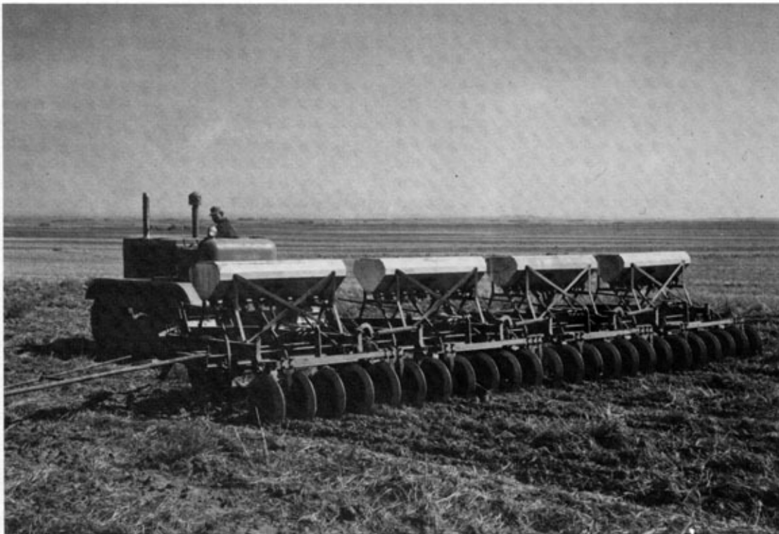
Fig. 124 Deep furrow drill seeding wheat on stubble-mulched field (USDA-Soil Conservation Service photo)
