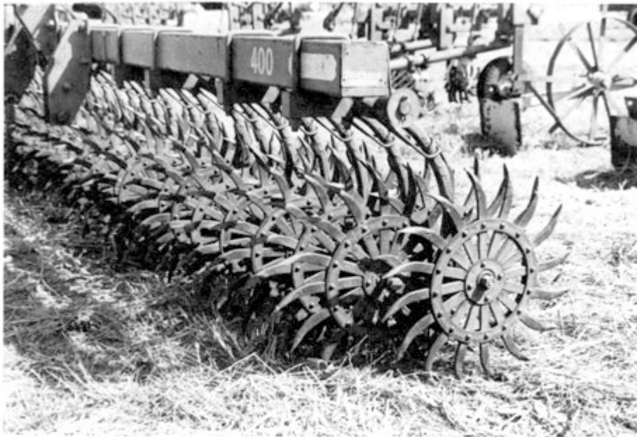
Fig. 80 Rotary hoe used to break surface crusts to enhance seedling emergence and to roughen the soil surface to control wind erosion
