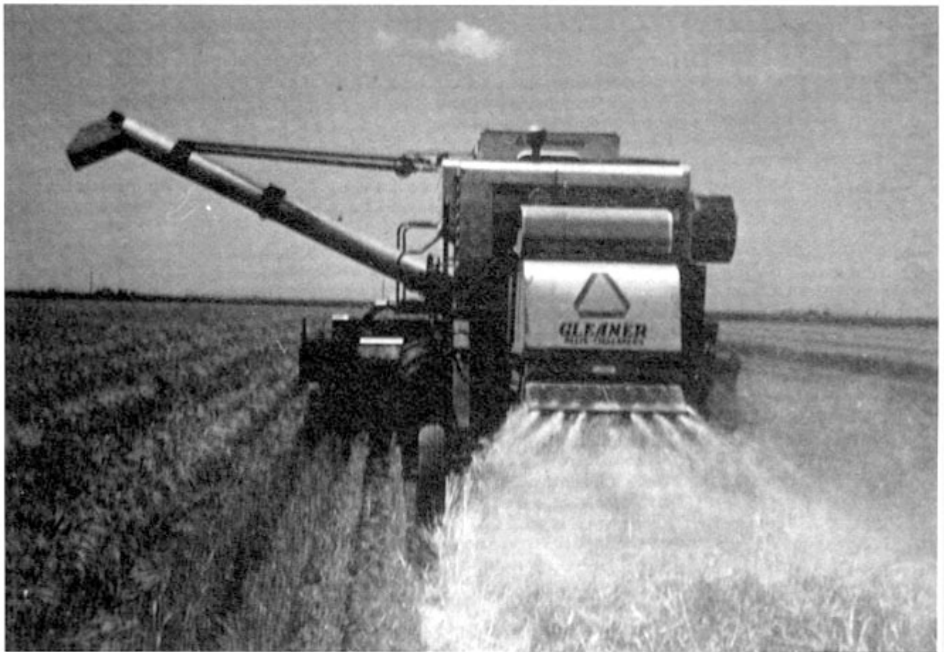
Fig. 83 Harvester equipped with straw spreading attachment: spreading the straw minimizes subsequent tillage problems
