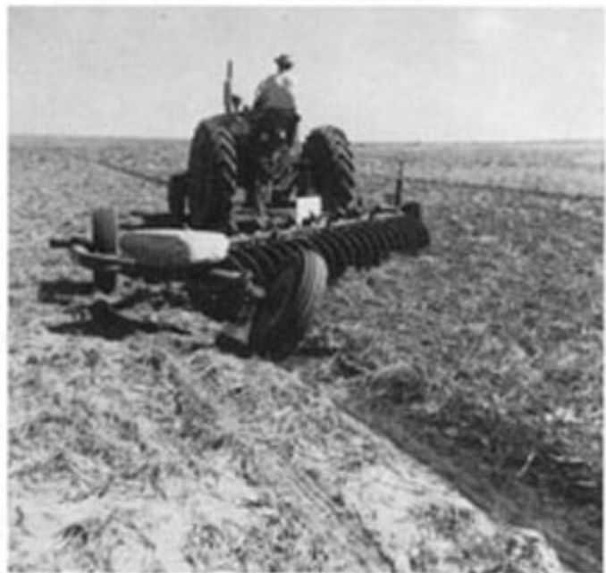
Fig. 40 one-way disk plough (photo provided by C.R. Fenster, University of Nebraska)
