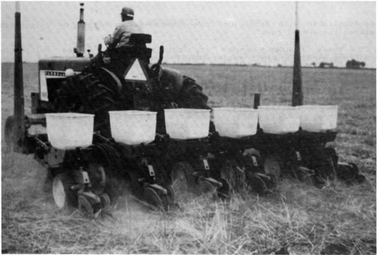
Fig. 132 Seeding sorghum in wheat residues with unit planters in no-tillage method
