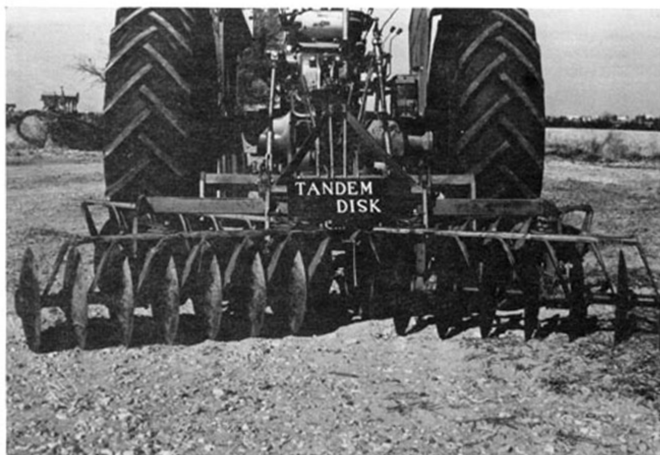
Fig. 65 Tandem disk harrow. Disk harrows pulverize dry soil and, therefore, can lead to water and wind erosion problems (photo provided by C.R. Fenster, University of Nebraska)
