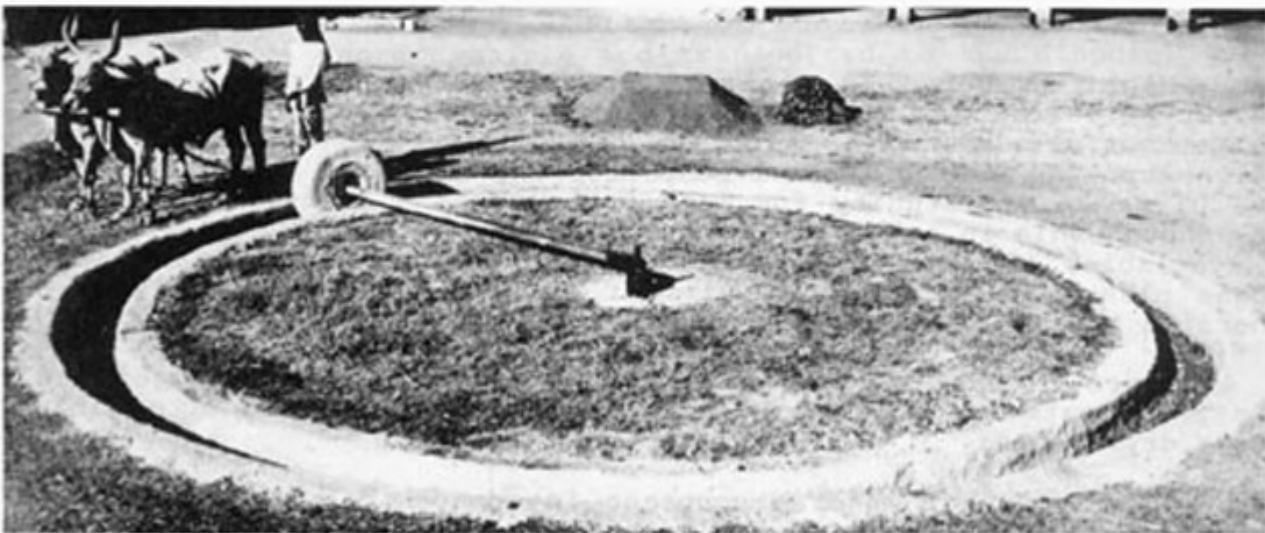
Plate 8 Crushing urine-earth from cattle sheds in a lime mortar mill Source: Howard and Wad (1931)
