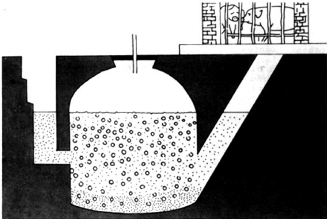
Plate 30 Biogas unit showing inlet from pig-sty, the digester and the sludge outlet pipe Source: FAO filmstrip Biogas in China
