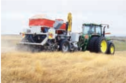
PLATE 32 No-till drilling a wheat crop into an erosion-prone field protected by herbicided pasture [BAKER NO-TILLAGE LTD]
