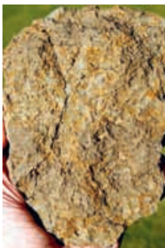
POOR CONDITION VS = 0 Soil has abundant to profuse (> 50%) medium and coarse orange and particularly grey mottles.
