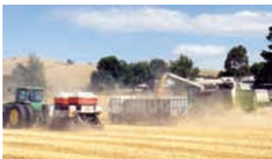
PLATE 34 Harvesting a wheat crop followed immediately by no-till seeding the next crop into stubble [BAKER NO-TILLAGE LTD]
