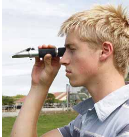
Assessing the sugar content (Brix) of pasture sap with a hand-held refractometer.
