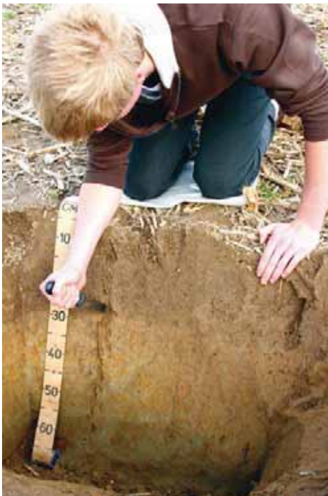
PLATE 17 Identifying the presence or absence of a hardpan with a knife
