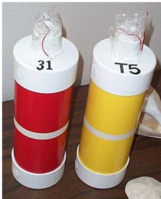
Figure 9.17. Float-out devices prior to installation. Color coded and numbered for identification purposes.
