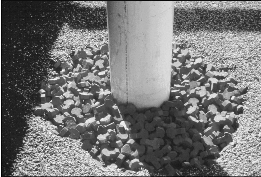
Figure 5.23. Laboratory study of Toskanes for pier scour protection.
