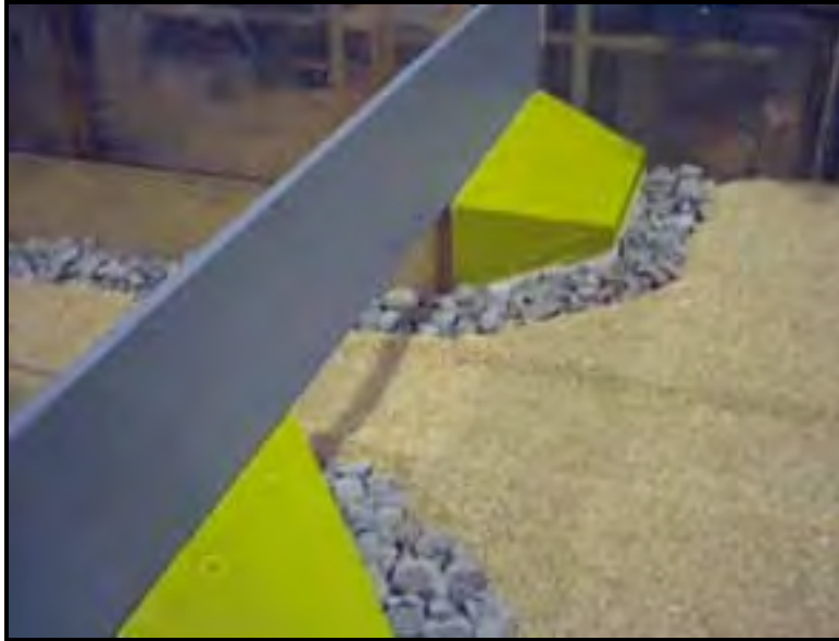
Figure 18.7. Riprap protection at a bottomless culvert with the MDSHA Standard Plan (Kerenyi et al. 2007).
