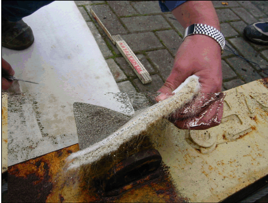
Figure 11.17. Close-up photo of SandMat™ geocomposite blanket. (photo from NCHRP Project 24-07(2), courtesy Colcrete – Von Essen Inc.)
