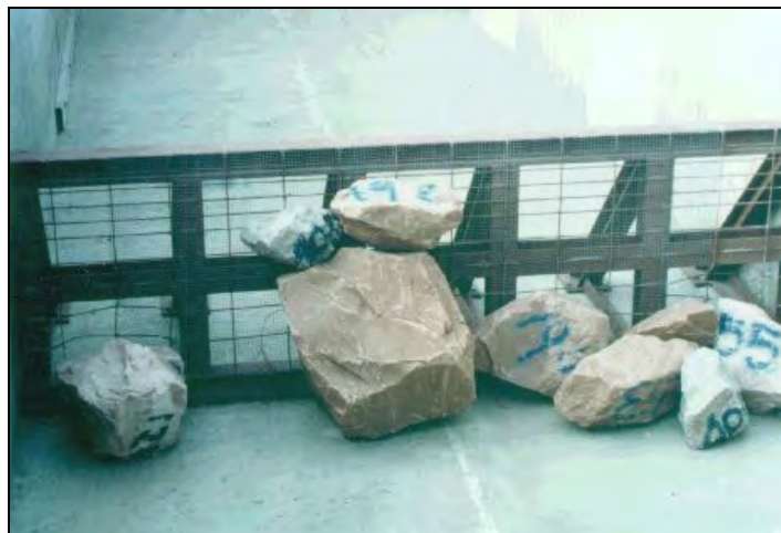
Figure 5.8. Failure of riprap in 1995 tests ( d_{50} = 2.15 ft (655 mm))
