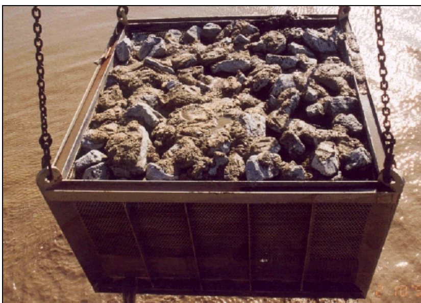
Figure 12.21. Test box used during underwater grout placement.
