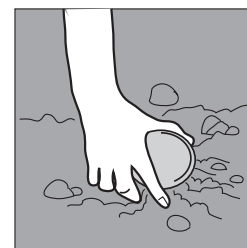
Figure 4, pushing sample can into soil
