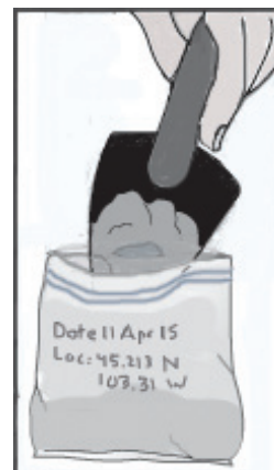
Figure 3, placing soil in zip lock bag
