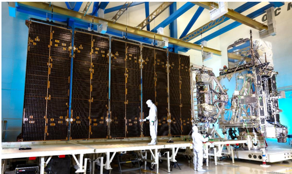
Figure 11-3. The Solar Array installed on GOES-16
