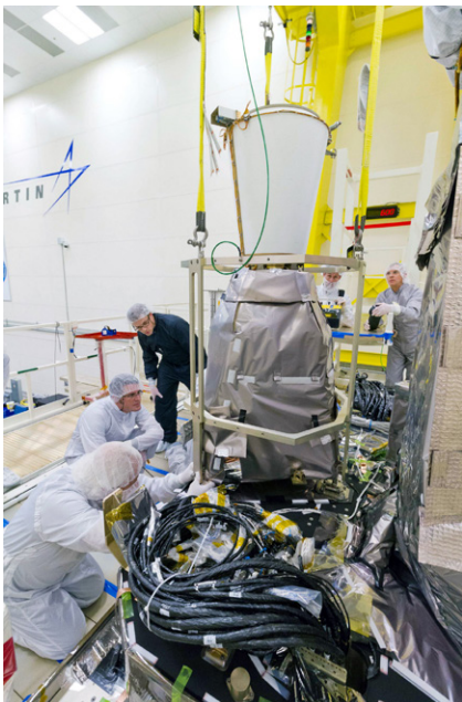
Technicians install the GLM on the GOES-R spacecraft. Credit: Lockheed Martin
