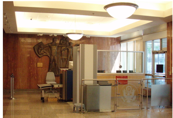
Figure 5.02 The ability to view artwork should be considered when dropping ceilings or making alterations. Although not a First Impressions project, this image was included to demonstrate design issues that can arise from architectural modifications in the vicinity of artwork. In this instance, the female figure's head is visually obscured when viewed from the lobby area by the dropped ceiling.
