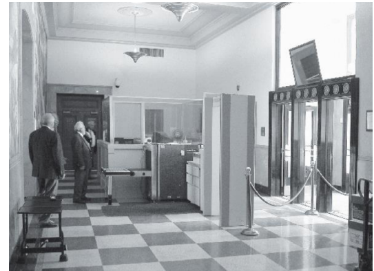
Figure 7.49 The security station strives to maximize queuing space and separate types of traffic.
