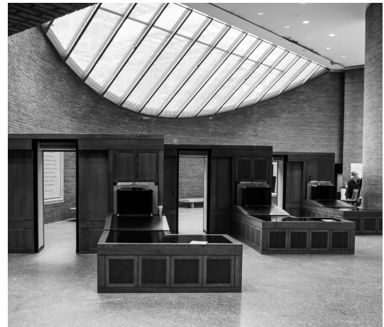
Figure 7.28 The use of wood and the detailing of the integrated security stations adds warmth to the space. In addition to up-front queuing space, the design also considers the space needed after security for bag pick-up and more detailed screening.
