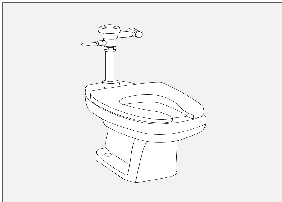
Figure 5-3. Flush Valve Toilet.
