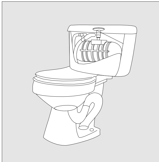
Figure 5-4. Pressurized Tank Toilet.
