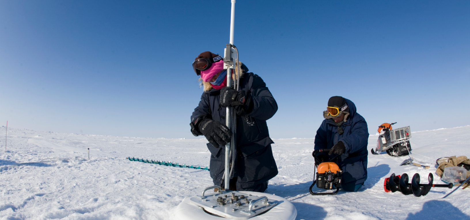
U.S. Army Corps of Engineers researchers Jackie Richter-Menge and Bruce Elder install an ice mass balance buoy in the Beaufort Sea. Photo: Art Howard, via DOD
