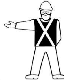
MOVE TAIL ROTOR Rotate body w/one arm extended
