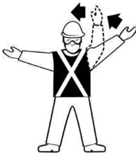
MOVE LEFT Right arm extended left arm sweeps overhead
