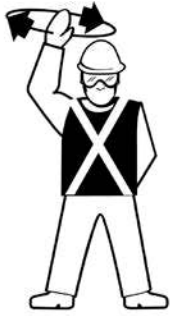
CLEAR TO START Make circular motion above head w/arm
