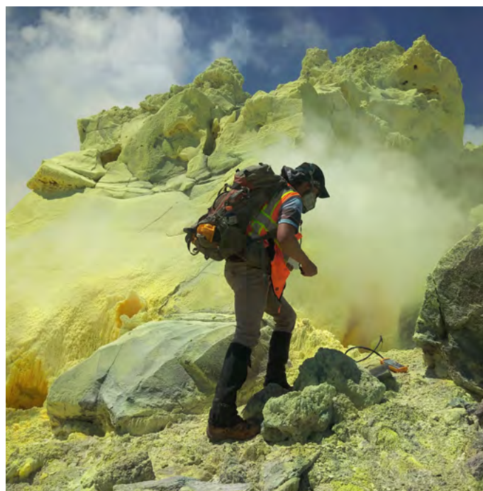
Gas sampling with MultiGAS sensor at Minas de Azufre sulfatara inside Sierra Negra volcano, Galapagos islands, 2022. Picture credit: Daniel Sierra
