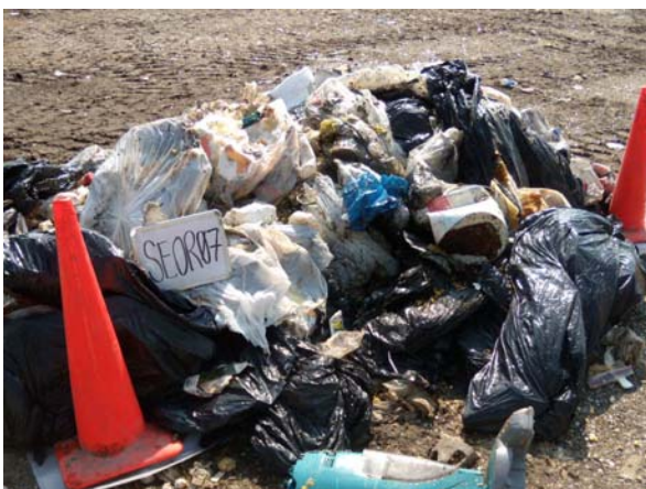
Figure 2-2 Example of a Grab Sample Staged for Manual Sorting
