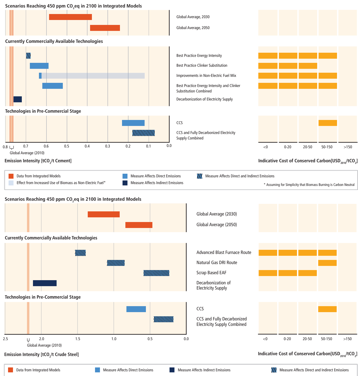
Figure TS.27 | Indicative CO 2 emission intensities for cement (upper panel) and steel (lower panel) production, as well as indicative levelized cost of conserved carbon (LCCC) shown for various production practices/technologies and for 450ppm CO 2 eq scenarios of a limited selection of integrated models (for data and methodology, see Annex III). DRI: Direct reduced iron; EAF: Electric arc furnace. [Figures 10.7, 10.8]
