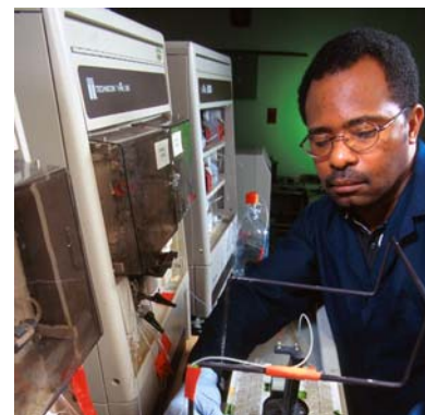
A flow-through colorimetric autoanalyzer is used to determine nutrients in shallow ground water. Photo by Scott Bauer(USDA-ARS).
