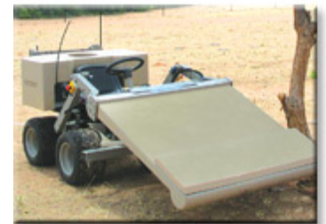
NIITEK Minestalker™ detects anti-tank landmines, explosives, and buried anomalies through remote subsurface visualization.
