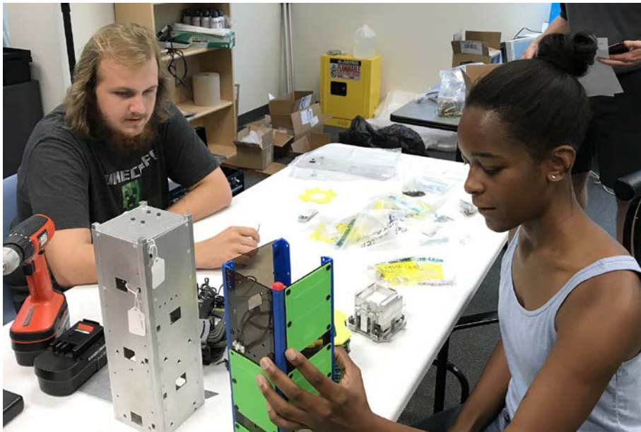
Students Jacob Hambur and Trisha Joseph from the University of Central Florida constructing the Q-PACE CubeSat. [University of Central Florida]
