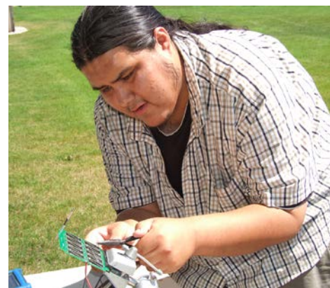
Salish Kootenai College student Zachary DuMontier tests solar panels on BisonSat . The BisonSat mission is an Earth Science mission that will demonstrate the acquisition of 100-meter or better resolution visible light imagery of Earth using passive magnetic stabilization from a CubeSat. BisonSat is the first CubeSat designed, built, tested, and operated by tribal college students. Launched by NASA's CubeSat Launch Initiative on the ELaNa XII mission as an auxiliary payload aboard the NROL-55 Mission on October 8, 2015. [Salish Kootenai College]
