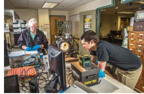
Denise Thorsen and Jesse Frey from the University of Alaska Fairbanks are performing DITL testing on the Alaska Research Center (ARC) CubeSat. ARC was launched by NASA's CubeSat Launch Initiative on the ELaNa XII mission as an auxiliary payload aboard the NROL-55 Mission on October 8, 2015. [University of Alaska, Fairbanks]
