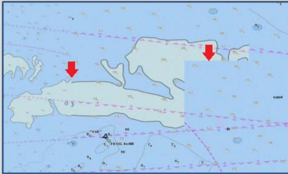
Figure 18 – This image shows three ENC cells. The extent of the 60 ft (18.2m) depth area in the ENCs on the left and center does not match. The ENC on the right does not show this depth area at all.
