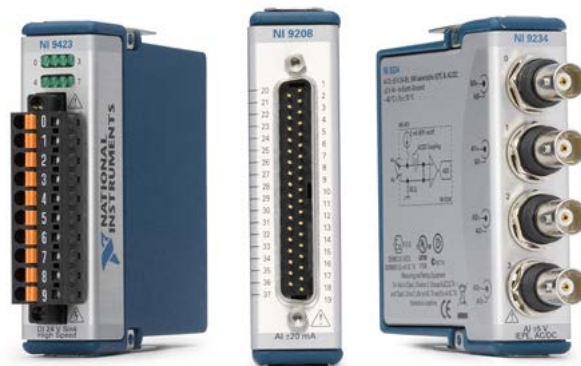
FIG 3 Add analog input, analog output, digital input, digital output, and some communication busses such as CAN and LIN to your CompactDAQ-based test system by installing C Series modules in available chassis slots.
