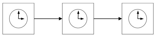
Grandmaster Clock This clock determines the time base for the system Slave to the Grandmaster Clock and Master to its Slave
