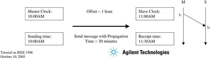
Send a message, (Delay\_Req message), from <u>slave</u> to <u>master</u> and measure the apparent time difference between the two clocks.
