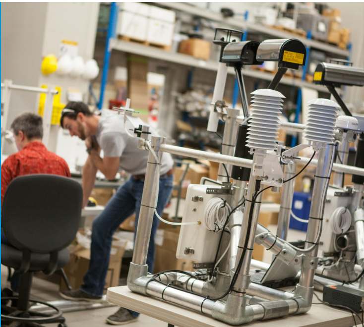
NSSL and academic partner employees calibrate instruments used for measuring tornadic wind speed and direction in preparation for deployment during VORTEX SE. (Credit: NOAA)
