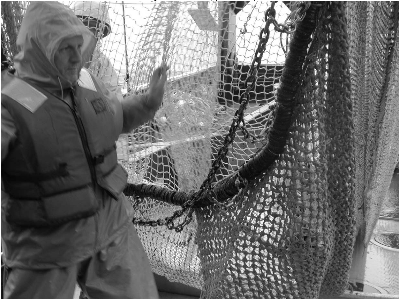
Exhibit 3. Canadian otter trawl showing details of wrapped footrope and tickler chain.
