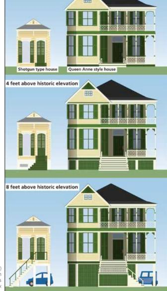
[76] Massing, scale, and proportions (tall vs. wide) are some of the important factors to consider when elevating a building and evaluating the impact on its historic character and appearance. *Graphic: Blank Space LLC for NPS*
