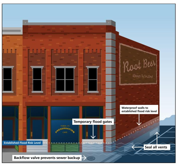
[47] Dry floodproofing is intended to keep all flood waters out of a building. This adaptation will include waterproofing walls, sealing openings, and installing backflow prevention devices. Any waterproof coatings should be carefully researched before applying them to historic wall surfaces and materials. *Graphic: Blank Space LLC for NPS*
