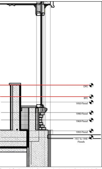
Figure 4: Section graphic of two-stage barrier at storefronts. Labels (from top to bottom) show the design flood elevation (DFE), base flood elevation (BFE), and various past flood events. *Drawing: KONTEXT architects Ilc*
