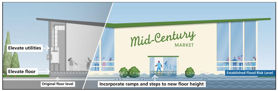
[100] Elevating the interior floor level above the established flood risk requires several building alterations, including constructing a new floor, elevating any utilities, and creating access to the new floor level. The original floor to ceiling height must be substantial enough to allow space for the new elevated first floor. *Graphic: Blank Space LLC for NPS*
