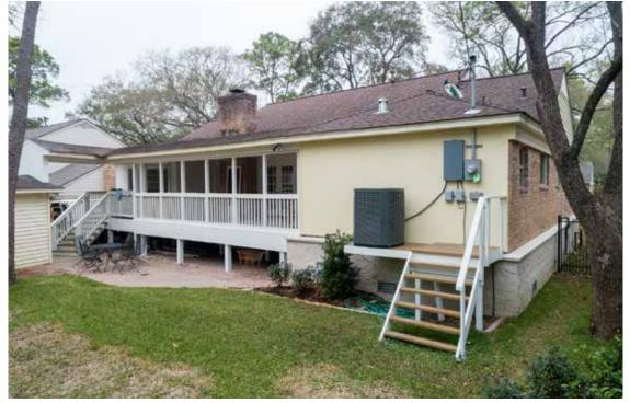
[44] Access issues must be considered when relocating exterior mechanical equipment on an elevated platform. If electrical or gas meters are moved to higher locations, stairs or a ladder may be required by the utility company to facilitate meter reading. Photo: p3elevation.com
