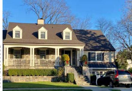
[93] This home has used elevated planting beds across the front of the house to bring the landscaping up higher and help screen the change in height. The stairs are stone, to blend in with the foundation and the planters, and a landing breaks up the long run of stairs at a point that aligns with the top of the planters. This provides a visual reference point for what was the original foundation height. The garage remains at grade level. Photo: FloodSavvy.com
