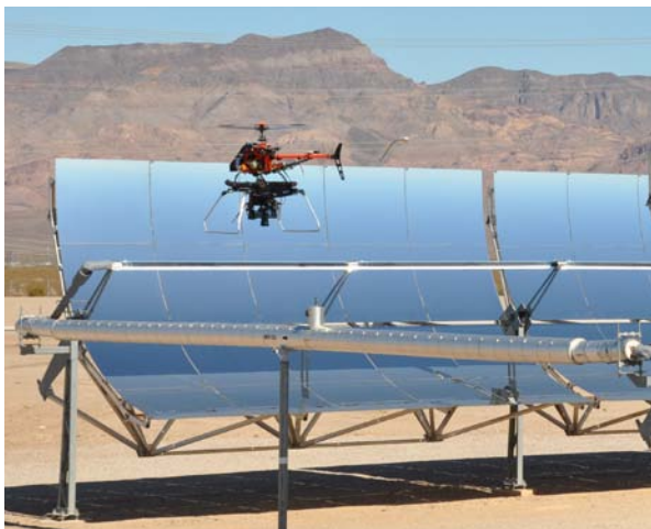
A high-performance radio-controlled helicopter, holding a specialized camera, is part of the Distant Observer photogrammetric data acquisition system. Here, the helicopter hovers over a trough in the Nevada Solar One CSP plant outside of Las Vegas. Photo by NREL Distant Observer Team, NREL/PIX 23115
