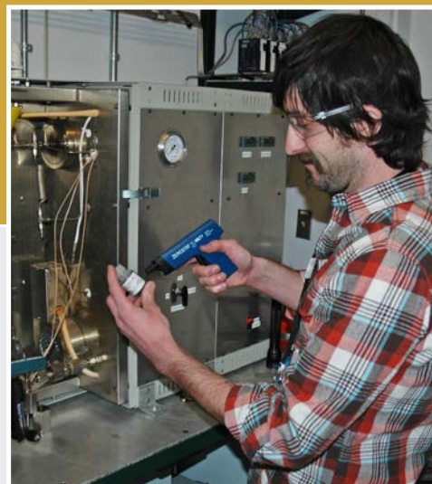
This bench-scale fuel synthesis reactor can be used to test various catalysts over a wide range of conditions using bottled or biomass-derived syngas. Photo by Jesse Hensley, NREL 19329
