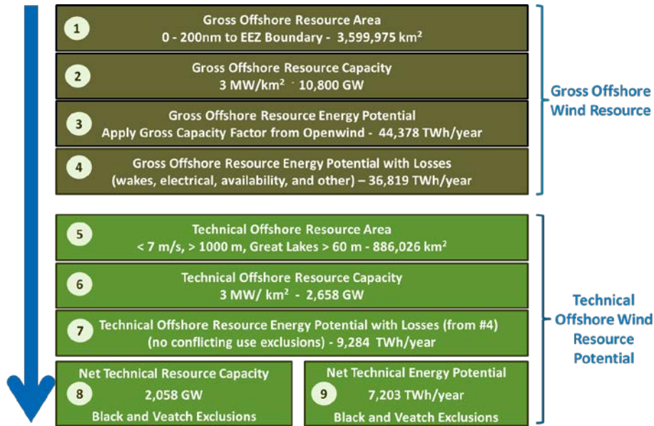
Figure ES-2. Progression of analysis for the 2016 Offshore Wind Energy Resource Assessment for the United States
