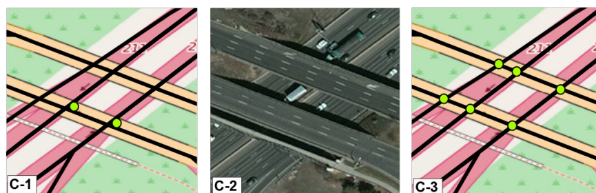
From left to right: C-1 is a screenshot of the original bridge point representation; C-2 is an aerial image of the bridge; and C-3 is a topologically corrected version of the bridge layer.
