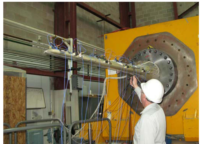
Low-pressure surface view of structural validation of the Verdant 56-kW Composite KHPS Blade at NREL. Photo by Mike Desmond, NREL 21715
