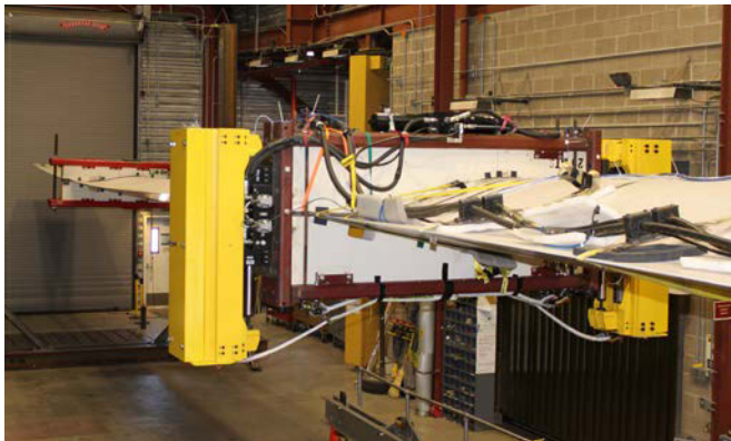
Biaxial fatigue assessment of an MHI Wind Power Americas, Inc. turbine blade at the NWTC. Photo by David Snowberg, NREL 28797
