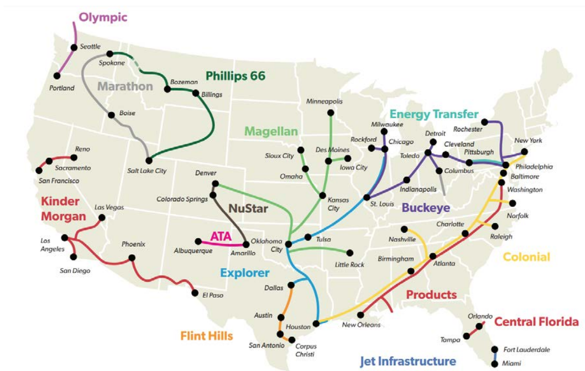
Figure 6. Major U.S. pipelines transporting jet fuel.
