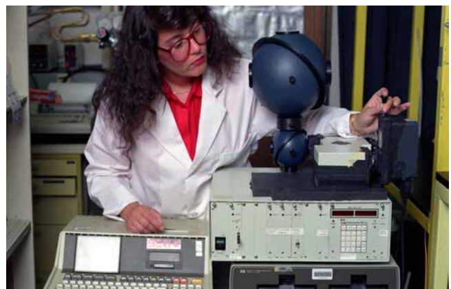
In 1990, Kim Magrini operates a device for measuring the output of high-intensity light sources. NREL Photo by Warren Gretz, NREL 03944
