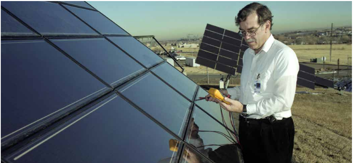
Keith Emery in 2001 at NREL's outdoor test beds to characterize the performance and reliability of PV cells, modules, and small (1-5) kilowatt systems. Photo by Warren Gretz, NREL 10750
