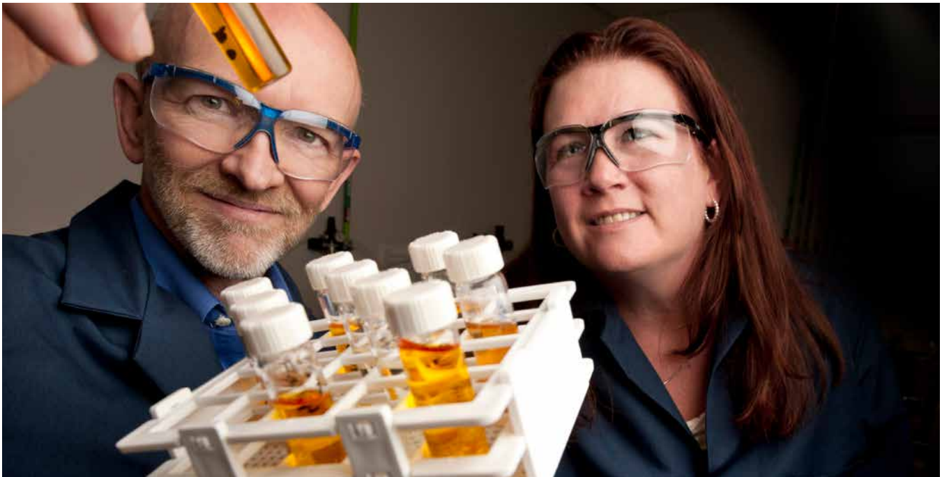
Robert McCormick and Teresa Alleman sorted a variety of chilled biodiesel samples in 2012 to be introduced to a mass spectrometer for analysis in the Fuels Performance Lab. Photo by Dennis Schroeder, NREL 21940
