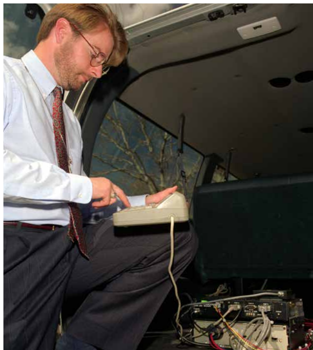
Keith Wipke installing transmitters and small computers on the shuttle bus in 1996 to streamline van pickups and deliveries via satellite relay. Photo by Warren Gretz, NREL 02292
