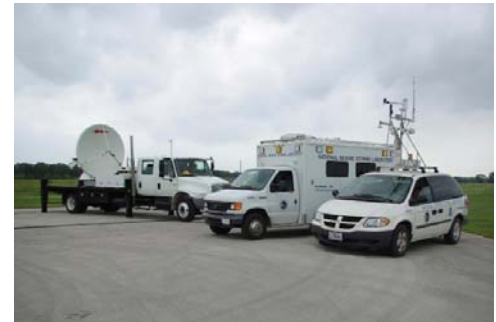
The NO-XP mobile radar (rear), mobile field command vehicle and mobile mesonet were deployed to collect data when Hurricane Ike made landfall on the Texas coast.
