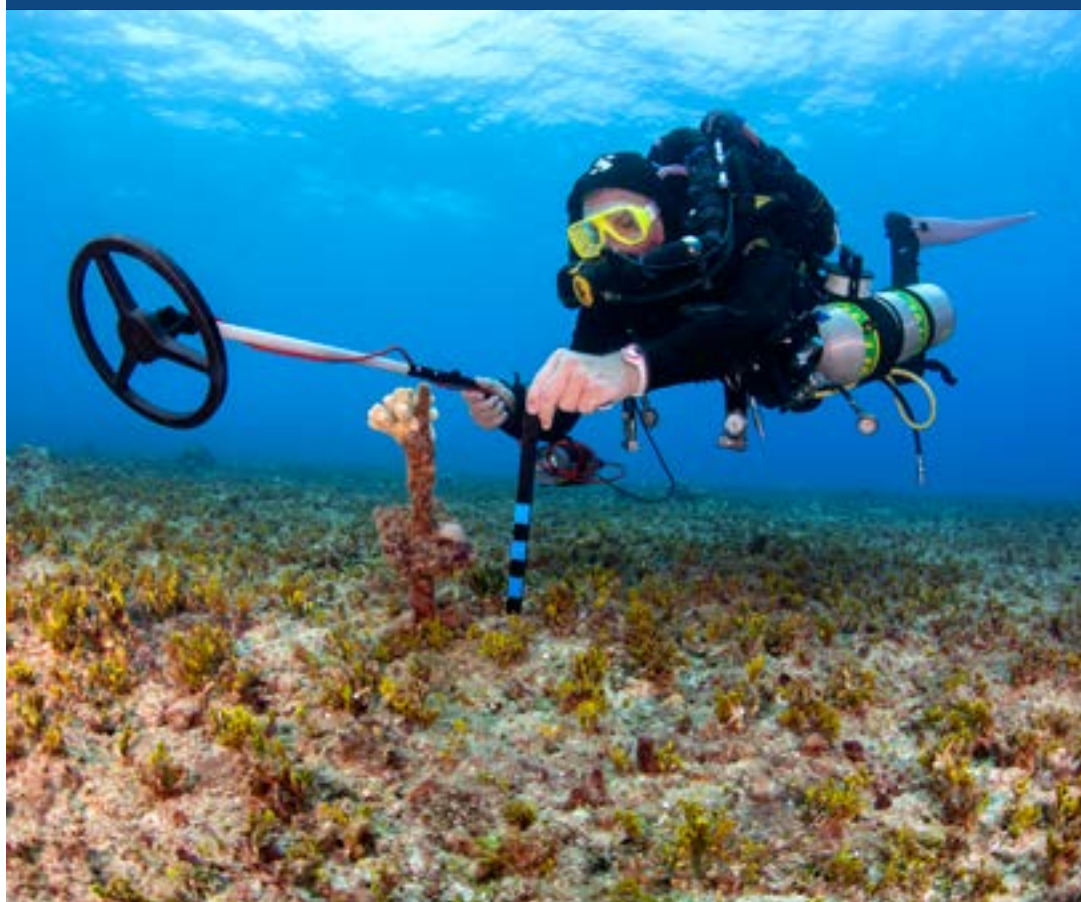
Below photos: a diver uses an underwater metal detector to find sunken artifacts.
