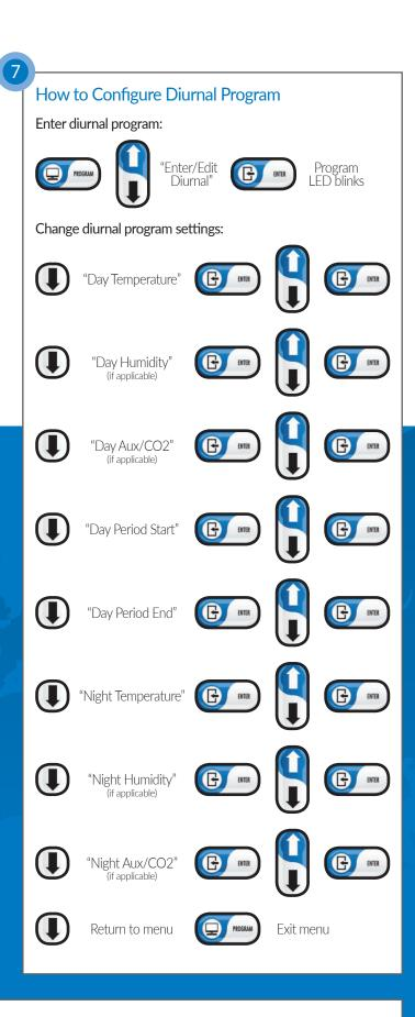
Programming Note: The controller will default back to the main display when no key is pressed after one minute. Please keep this in mind when programming the controller. Problems? Questions? Refer to the IntellusUltra controller manual for more instructions. Contact us for additional support.
