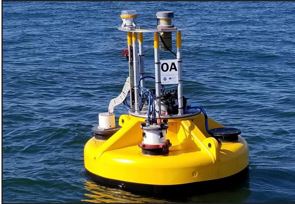
A buoy used to monitor the changing chemistry in the Chesapeake Bay. Credit: NOAA
