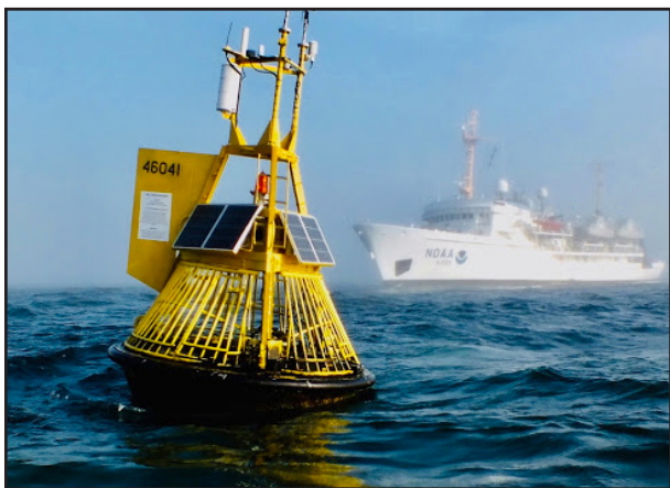
An ocean acidification buoy located off the central Washington coast is serviced by researchers aboard the NOAA Ship Fairweather in 2012. Credit: Richard Feely/NOAA
