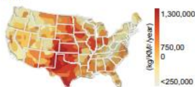
B: Hydrogen production potential from utility-scale PV, by county land area
