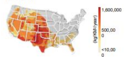
C: Hydrogen production potential from concentrated solar power, by county land area
