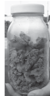
図6 DME脱水後の下水汚泥 Fig.6 Dewatered sludge cake by DME
