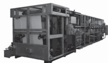
図11 実機外観 Fig.11 Appearance of Squeeze and Blow Dehydrator
