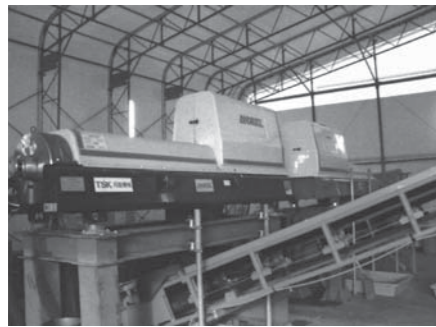
図6 仮設脱水機運転の状況 Fig.6 Operational condition of the temporary dewatering machine
