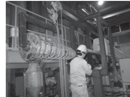
図15 現地分解の様子 Fig.15 The situation of disassembling decanter on site
