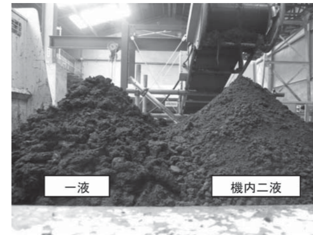
図7 脱水ケーキの外観比較 Fig.7 Comparison of cake in appearance (Polymer flocculant conditioning vs Two-flocculant conditioning)
