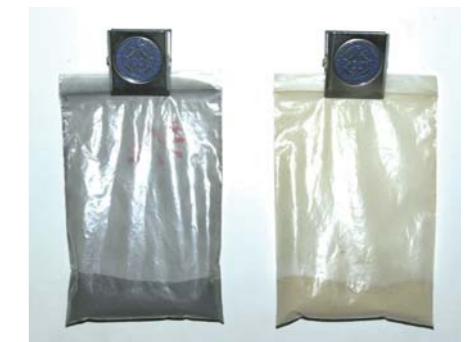
図4 石炭の常圧FBCとPFBCでの灰の比較 左：常圧、右：加圧 Fig.4 Photograph of ash produced by FBC and PFBC. Left: Atmospheric condition. Right: Pressurized condition (0.8MPa).
