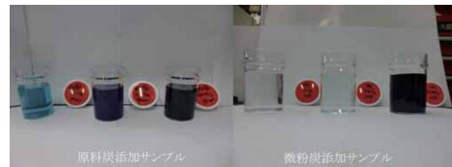
図6 メチレンブルー脱色後の写真(活性炭添加率:左から0.1%・0.05%・0.005%) Fig.6 Pictures of methylene blue adsorbed on PAC and S-PAC (Additive rates of activated carbon : 0.1%, 0.05%, 0.005% left to right)
