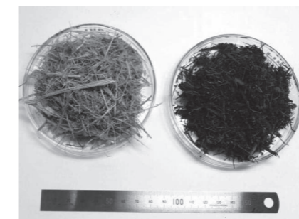
図4 クラッシング開始直前(右)と直後(左)のバガスの写真 Fig.4 Photo of bagasse (Right: old and degraded bagasse. Left: newly crushed and fresh bagasse.)
