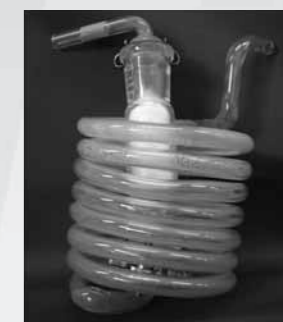
図2 排ガス採取後のスパイラル管の全体写真 Fig2 Whole view of spiral tube after collection of exhaust gas
