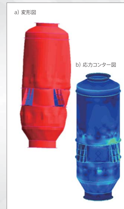
図3 燃焼炉解析結果 Fig3 Analysis results of combustion furnace
